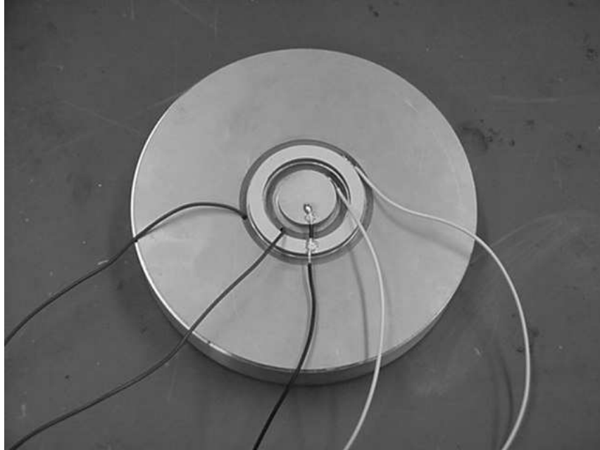
Figure 3.17 The rear actuators of mirror S2.
