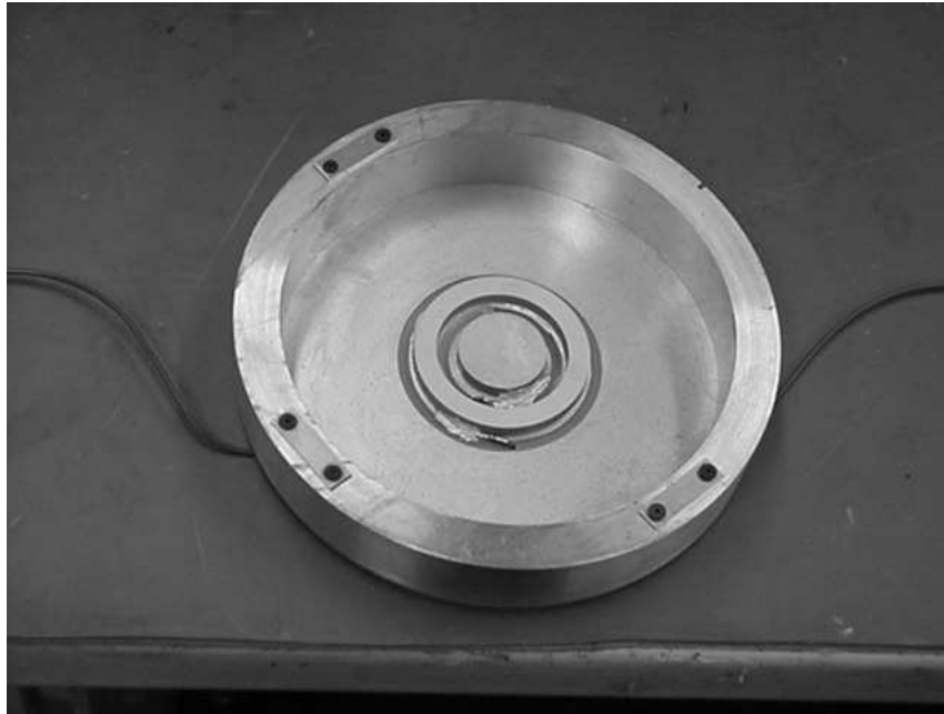
Figure 3.16 The interior actuators of mirror S2.
