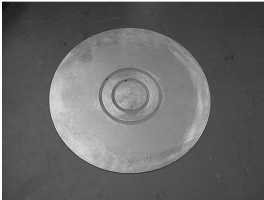
Figure 3.15 The copper baseplate used for mirror S2.
