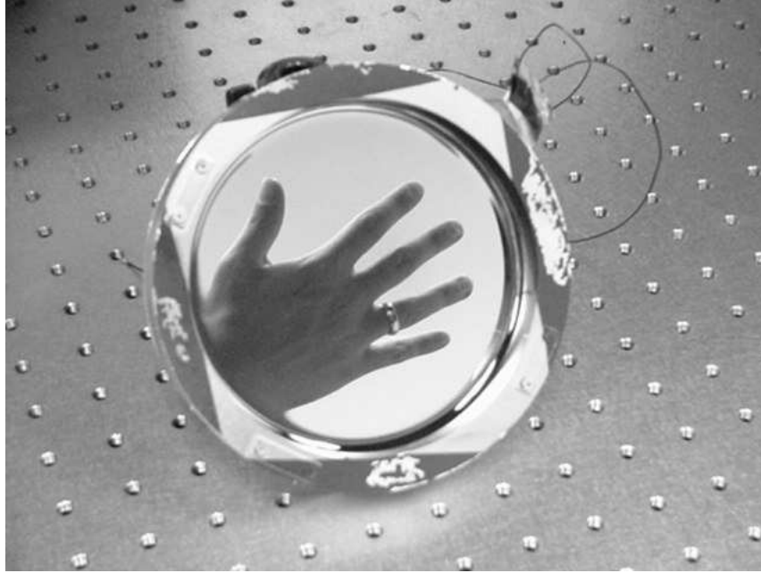
Figure 3.10 M1 after a reflective layer of gold has been applied.
