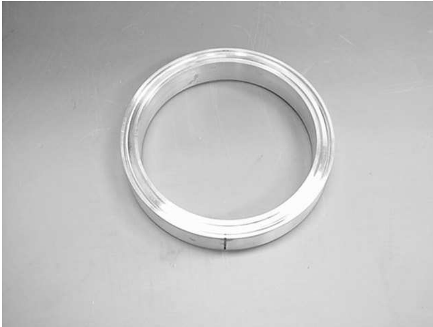
Figure 3.3 The 6" diameter membrane mounting ring.
