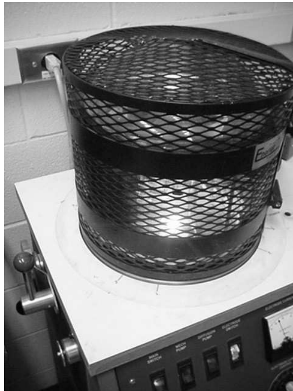
Figure 3.9 The glowing heating element is visible during the gold evaporation process.
